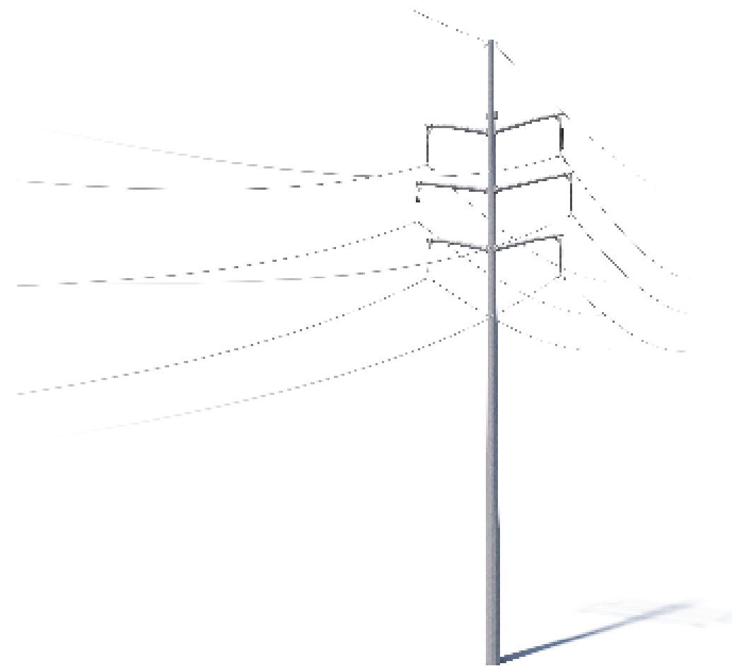
The project involves building a new transmission line with double-circuit steel monopole structures.
